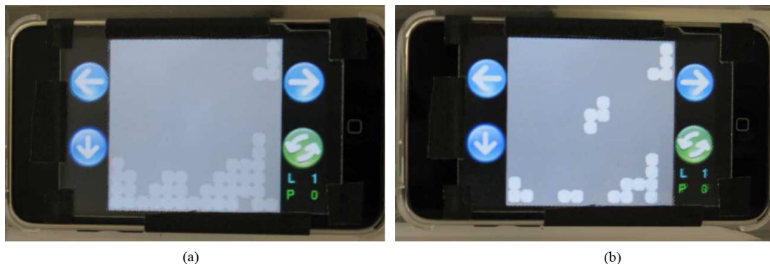
Fig. 4. The game prototype using an iPod Touch with an overlay lenticular lens, which provides different content to each eye. The two pictures are presented simultaneously, but each is only visible to a specific horizontal viewing angle. (a) View to the fellow eye: All the information sent to the fellow eye is in low contrast. Static Tetris blocks buried below other blocks at the bottom of the gameboard are fully visible. (b) View to the amblyopic eye: All the information sent to the amblyopic eye is in high contrast. The falling Tetris is visible, as are some of the buried blocks at the bottom of the gameboard.
