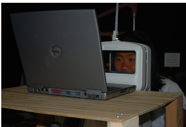
Figure 1 Photograph of the experimental setup shows the laptop computer positioned in front of the infrared optometer. The colored filters, required for measurement of AP, are not shown here.
