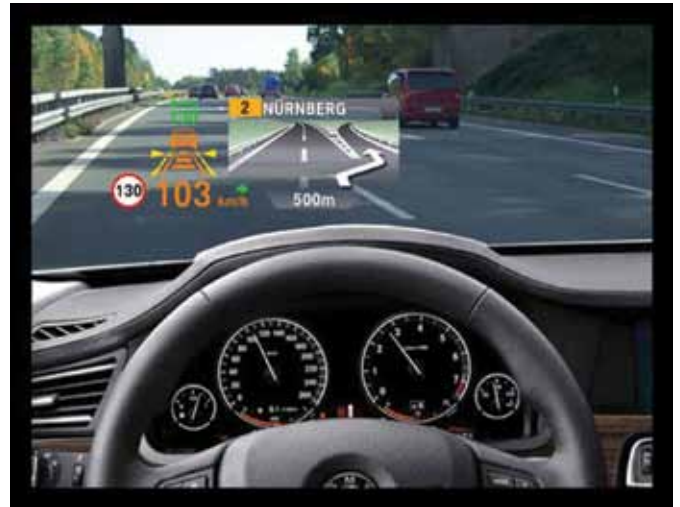
Figure 2. Head-up displays, as shown, are becoming more common in a wide range of cars (image from http://techdrive.co/2014/11/finally-time-head-displays-cars/s ).
