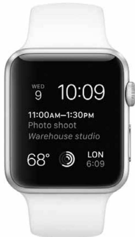
Figure 3. Wrist-mounted displays such as the Apple Watch (Apple, Cupertino, CA) may present other issues due to the limited screen area (approximately 3.3 × 4.2cm).
